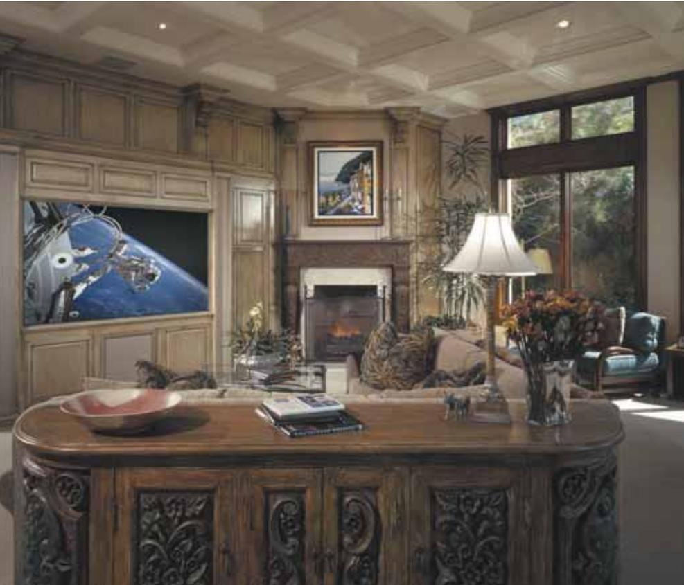
**In more classical environments, you can create a coffered ceiling system and fill the areas between the coffer beams with fabric and acoustical absorption.**
